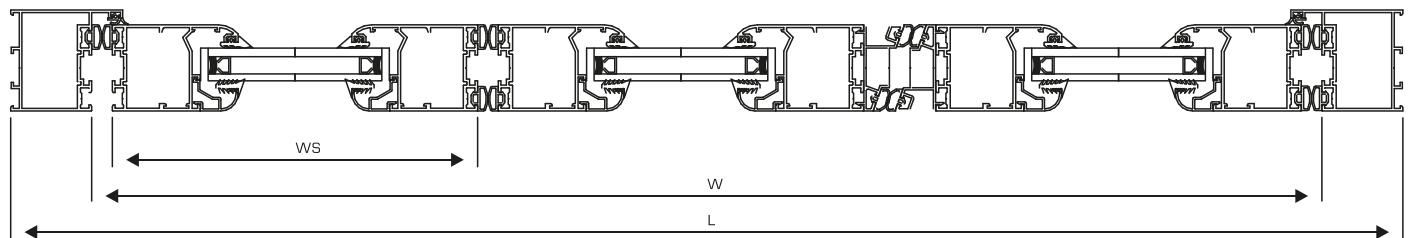
$$WS = \frac{(W - 44 \text{ mm}) - (N \times 12 \text{ mm})}{N}$$
