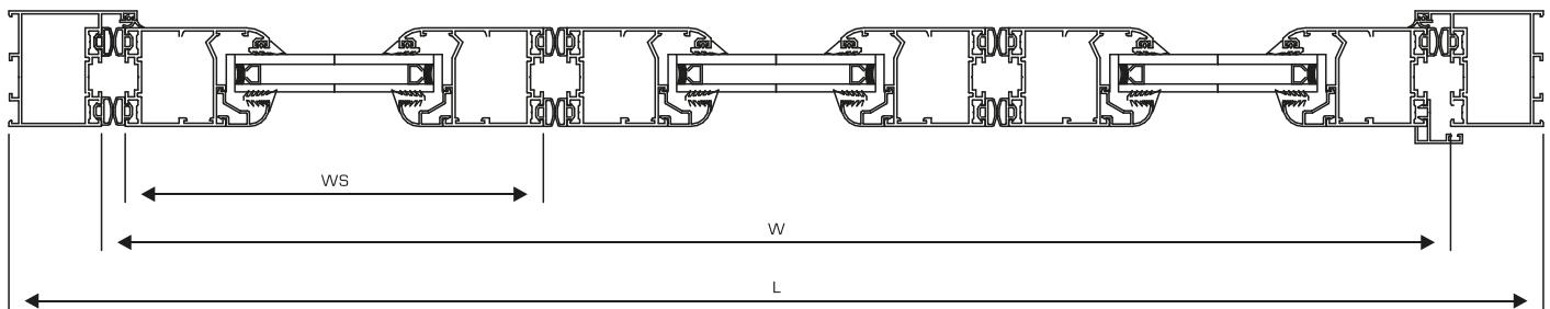
$$WS = \frac{(W - 12 \text{ mm}) - (N \times 12 \text{ mm})}{N}$$
